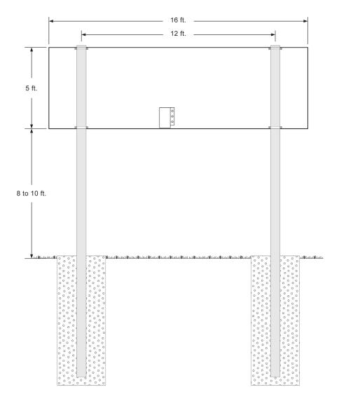
Once you have verified the positions of the posts and the size of the footings, you are ready to dig your holes, pour your concrete, and set your posts. There are several techniques for ensuring proper alignment of the posts. Typically installers will construct a temporary wooden support frame to hold each post in place while the concrete sets. Having plumb posts in the proper position is the key to a smooth mechanical installation.
